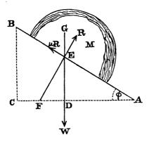
body M, whose weight is W, is just on the point of sliding down the plane, F the friction, and R the reaction of the plane on the body; then, resolving the forces which act on M along and perpendicular to the plane, we must have, for equilibrium,
